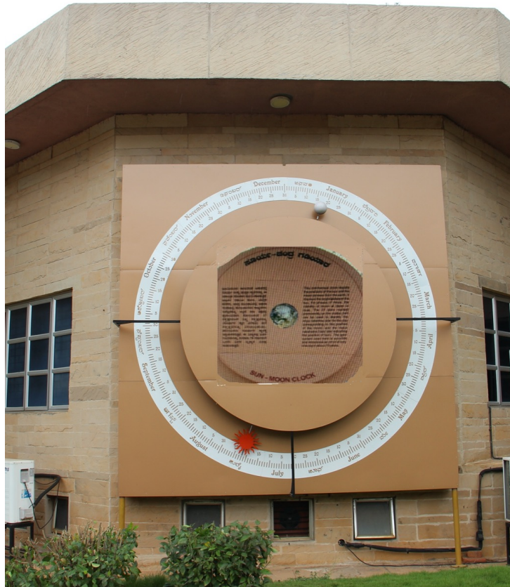
This clock depicts the position of the sun and the moon as well as the lunar phase.
